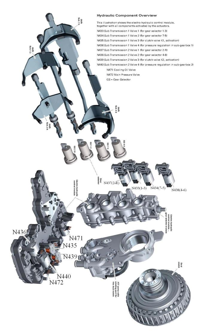
The 02E(DQ250),0BH(DQ500) and 0B5(DL501) are adaptive learn transmissions. The TCM can adapt the upshift and downshift pressure for each shift as well as the initial engagement into drive and reverse. Whenever the transmission is rebuilt or the valve body is changed, the shift adapts should be cleared and the vehicle should be driven to relearn the new adapts.
